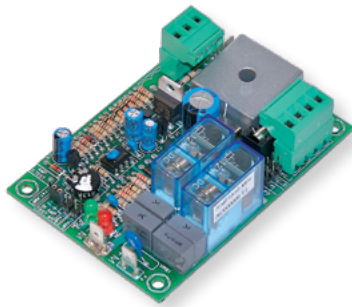
Control board - 2 channel | 2 Kanal - Motorsteuerung
